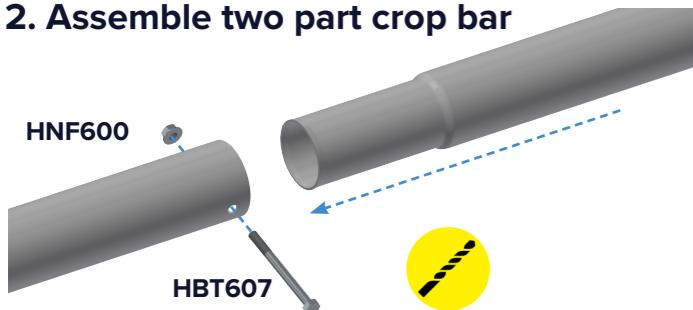
Connect two part crop bar. Drill and secure with nut and bolt.
