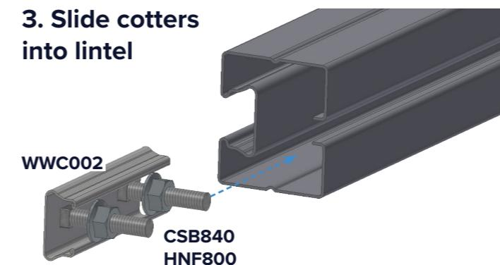
Slide two coppers into the lintel at each position **b**. Also slide two coppers at each position **c**. We'll use these for the door posts later.
