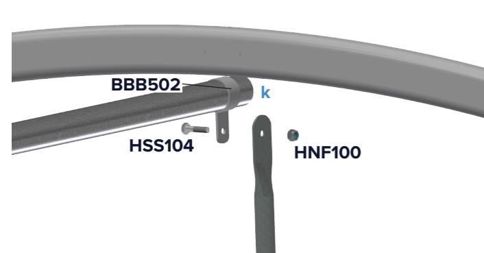
Attach single dropper to ridge bar with bracket.
