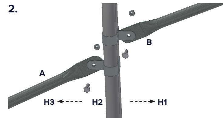
Note bracket configuration for brace bar **A** & **B** on hoop **H2**.
