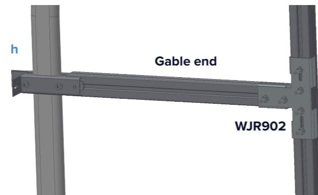
Attach gable end side rail to upright at position **d** using a T bracket. You should have two loose cotters in the upright from an earlier step.
