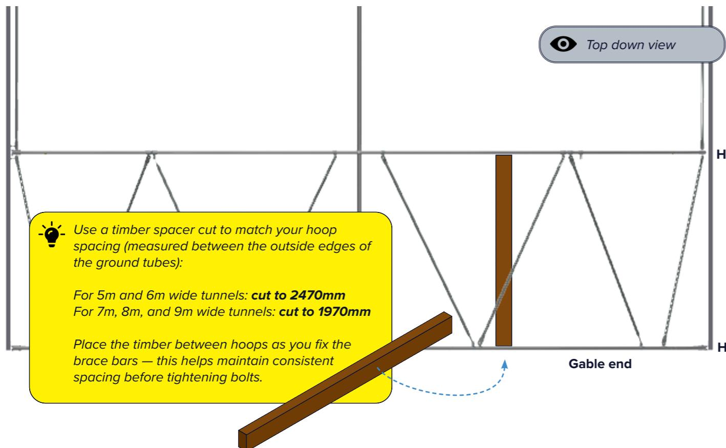
Ensure all hoops are vertical before fully tightening up. Fix brackets to hoops with tek screws.
