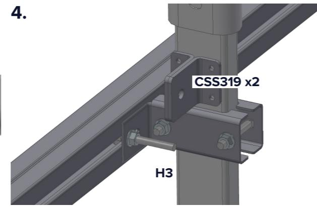
Note hoop **H3**. Attach bracket with tek screw and bolt brace bar **A** to bracket.
