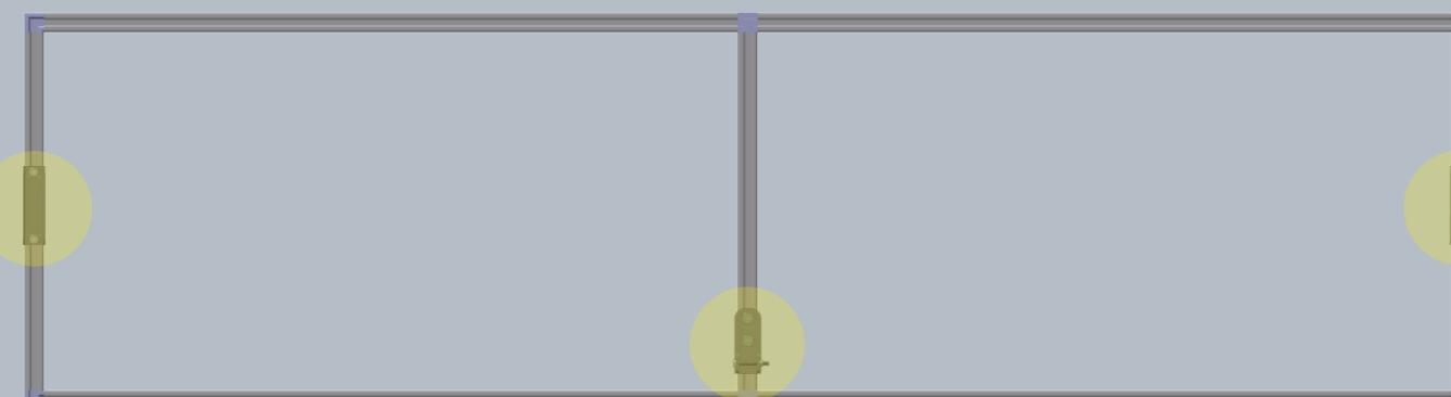
Roughly position brackets (highlighted) and leave finger tightened to allow for adjustment.
