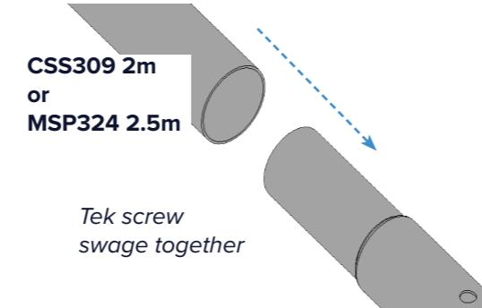
For each inner hoop, connect a length of ridge tube (CSS309)...
