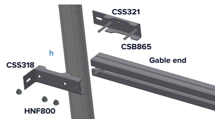
Attach gable end side rail to hoop using a side rail bracket. **Only on sides with side rail.**
