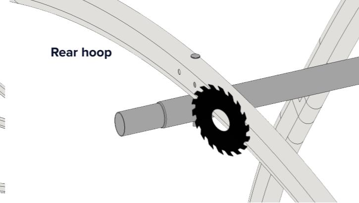
On the rear hoop, cut the protruding ridge bar flush with the outer face of the hoop. Insert plug RPP50.
