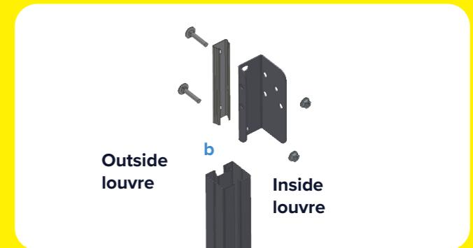
Install bracket to each H frame upright. Ensure correct orientation.
