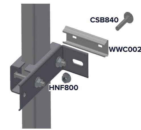
4. Slide base rails onto corner brackets
