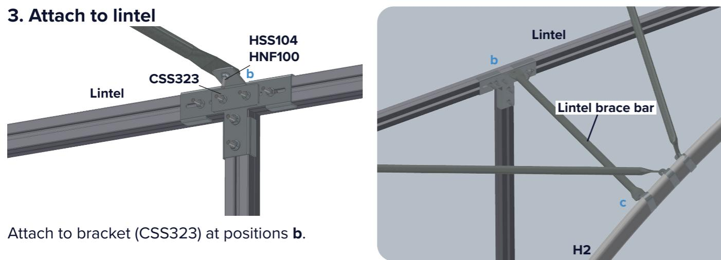
Attach to bracket (CSS323) at positions **b**.
