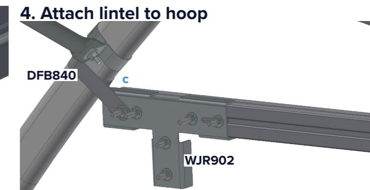
Attach the lintel to the hoop using a T bracket at positions **c**.
