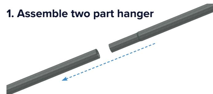
Connect two part hanger. Secure with a tek screw.
