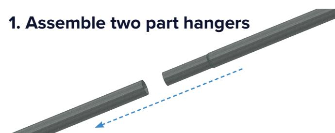
Connect two part hanger. Secure with a tek screw.
