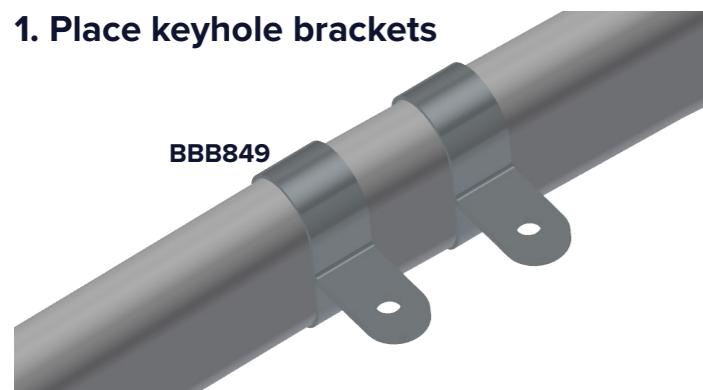
Place keyhole brackets on hoops. Splay the bracket to slide over the hoop.
