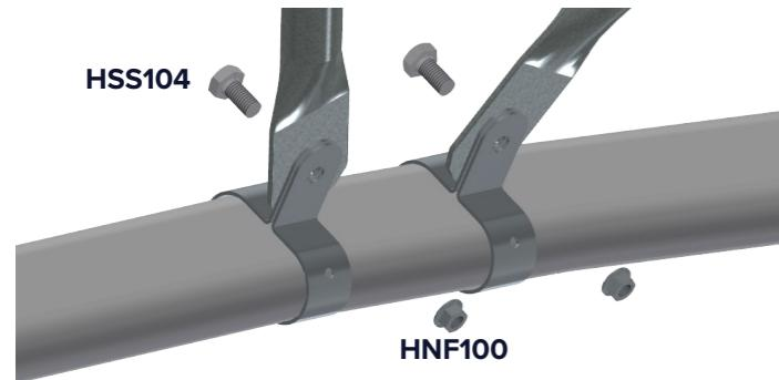
Attach brace bars to key hole clamps with nut and bolt.
