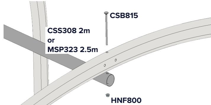
Starting at the front hoop, attach first ridge bar piece (CSS308) to hoop using nut and bolt.
