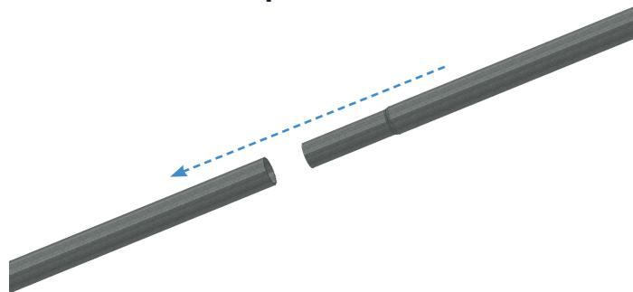
Connect two part lintel brace bar, and secure with a tek screw.
