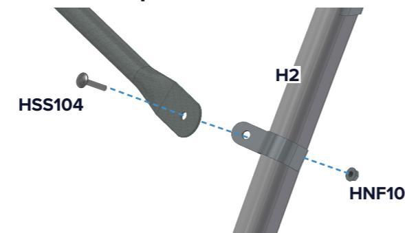
Attach lintel brace bar to hoop **H2**.
