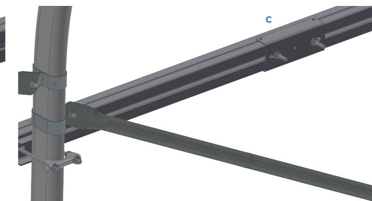
Tighten side rail to form a continuous side rail the full length of the tunnel.
