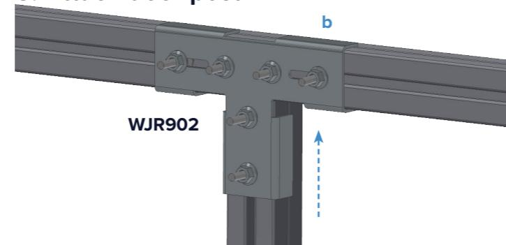
Attach door post to lintel at position **b** using a T bracket. Sink the bottom end into the 500mm foundation hole.
