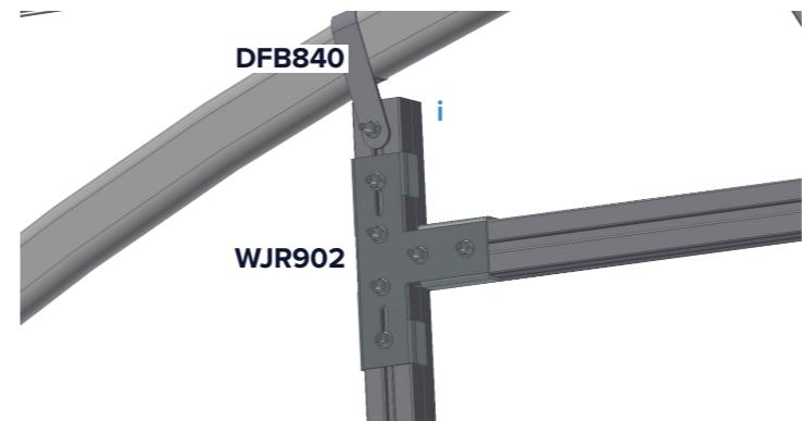
Install H frame configuration with T bracket at positions **i**...
