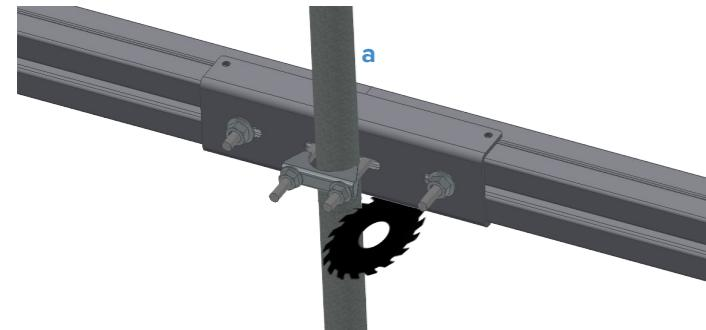
Then cut single dropper flush with the underside of the lintel.
