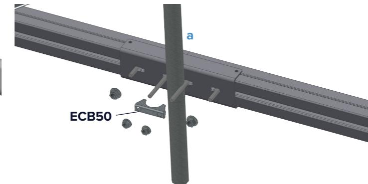
Attach single dropper to lintel with exhaust clamp.
