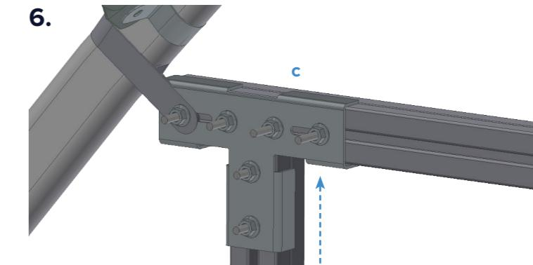
Attach the outer upright to the lintel at positions **c**. Sink the bottom end of profile into the 200mm foundation hole.
