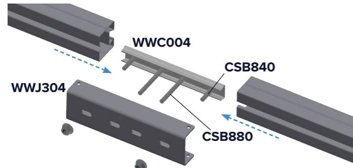
Join lintel using bracket (position **a**). If your structure includes louvres replace inner two bolts with short bolts (CSB840).
