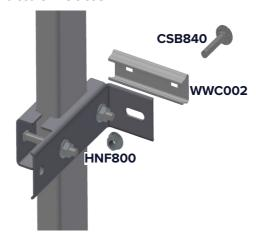
4. Slide base rails onto corner brackets
