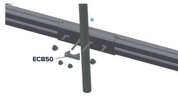
Attach single dropper to lintel with exhaust clamp.
