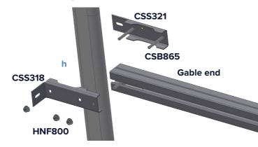
Attach gable end side rail to hoop using a side rail bracket. **Only on sides with side rail**.
