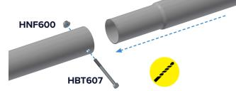
Connect two part crop bar. Drill and secure with nut and bolt.
