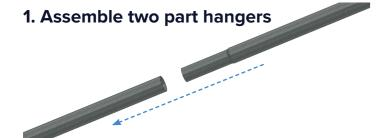
Connect two part hanger. Secure with a tek screw.
