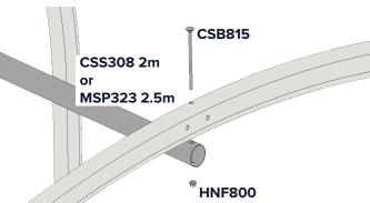
Starting at the front hoop, attach first ridge bar piece (CSS308) to hoop using nut and bolt.
