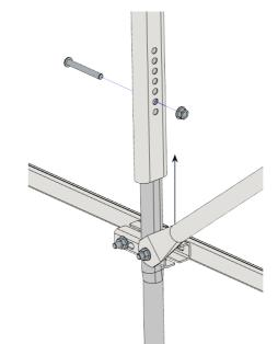
**10.** LIFT THE INNER HOOPS ONE AT A TIME TO TENSION THE COVER
