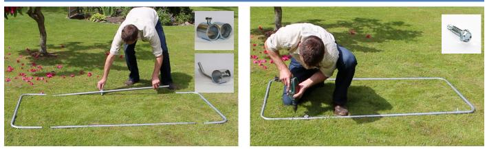
Slide two door hinges on one side and door latch on the opposite side. Fit sections of door together. In each corner drill a hole and secure with a self-tapping screw.
