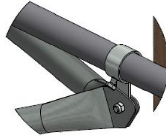
DETAIL ON 'E' BBB501 behind first and second hoop to take gable bracing
