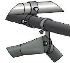
DETAIL ON 'D' BBB501 behind first and second hoop to take gable bracing
