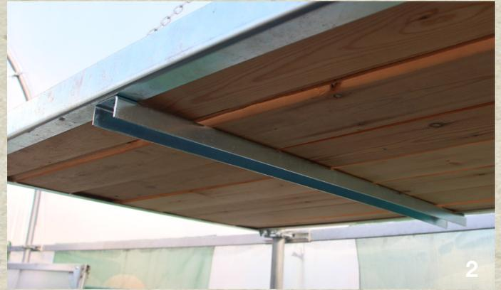
Line up the the steel sides and ends, ensuring the L-shaped side bar is fastened beneath the front end and rear bars (see image 1). Secure in place with the bolts provided. Please note: the images show the wooden slats already in place, this is for illustration purposes only, the slats are to be fitted in the last step.
